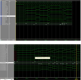
In above mentioned wave form March SS modelsim simulated wave has been shown, which is maintained in the idle state unless BIST\_En signal is made equal to 1. Hence all remaining operation is also performed as expected earlier.
